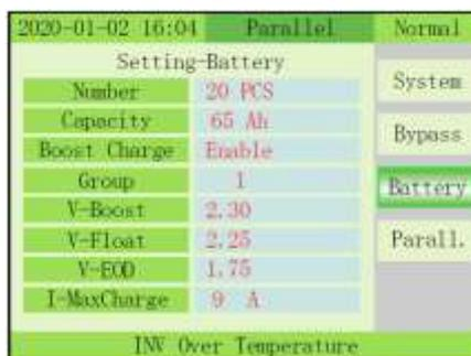
Fig. 4-14 Menú Setting/Maintenance - Battery
