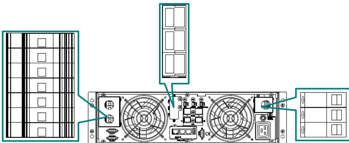
Fig. 5-1 Izda: Entrada tierra, Neutro Bypass, Neutro red, Bypass L, Red A (L1), Red B (L2), Red C (L3)
