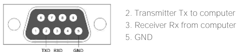
Fig. 5-3 RS232 communication port
