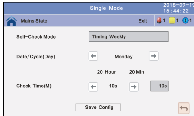
Fig. 4-20 Submenú Maint/Battery Self-Check/Timing Weekly
