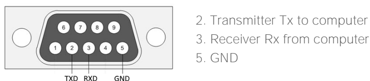
Fig. 5-3 RS232 communication port
