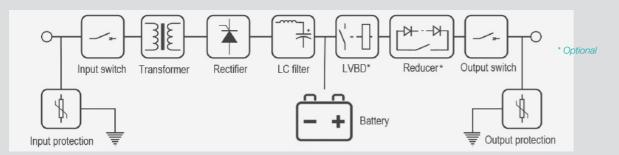
The power supply of the equipment is performed by direct connection to the AC current grid (50 Hz/60 Hz), either 230 V single phase (MIT1) or three-phase 400 V (MIT3). Also other nominal values on demand.
