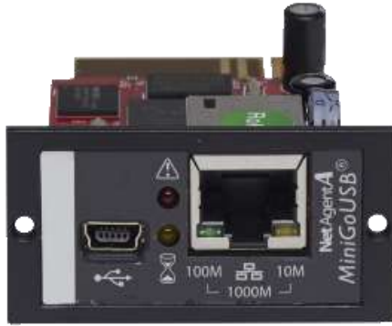
Fig. 5-5 SNMP/Modbus card view
