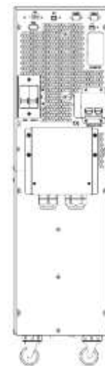
Fig. 2-3 Rear panel ZGR TOWER PRO 6 – 10 KVA (internal batteries at bottom section)
