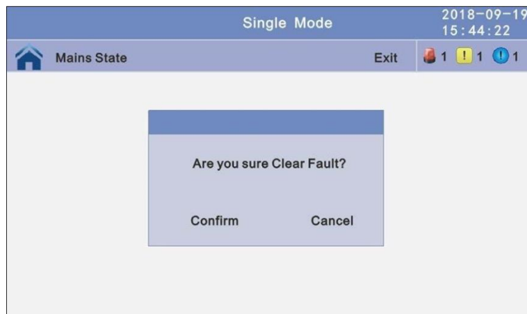
Fig. 4-58 Common/Fault Clear submenu
