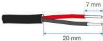
Fig. 4-45 Strip the protection layer
