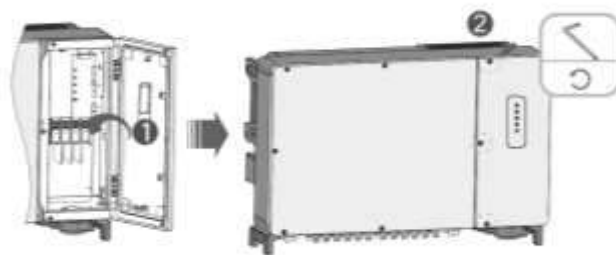
Fig. 4-49 Closing wiring compartment
