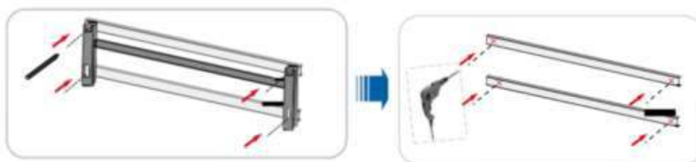
Fig. 4-11 Level the assembled mounting-bracket and mark the positions for drilling holes
