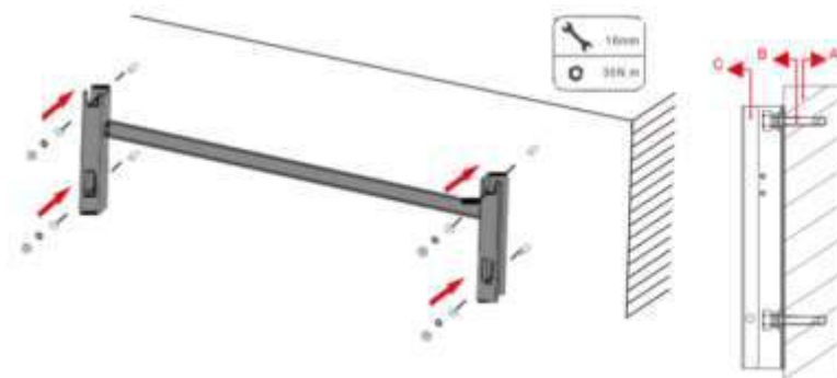
Fig. 4-18 Fix the mounting-bracket
