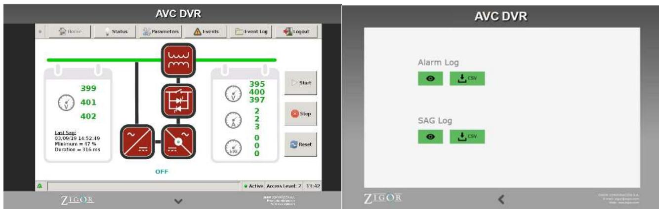
**Fig. 5-3 Monitoring and Download of Alarm and Sag Log**
