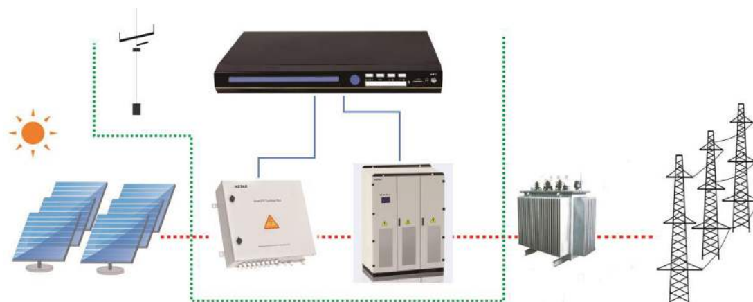
Fig. 2-1 Grid-tied PV Power Generation System composition
