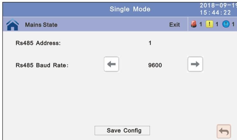
Fig. 4-28 Submenú Settings/Basic Settings/Communications
