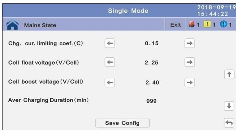
Fig. 4-37 Submenú Settings/Advanced Settings/System Setting (7)
