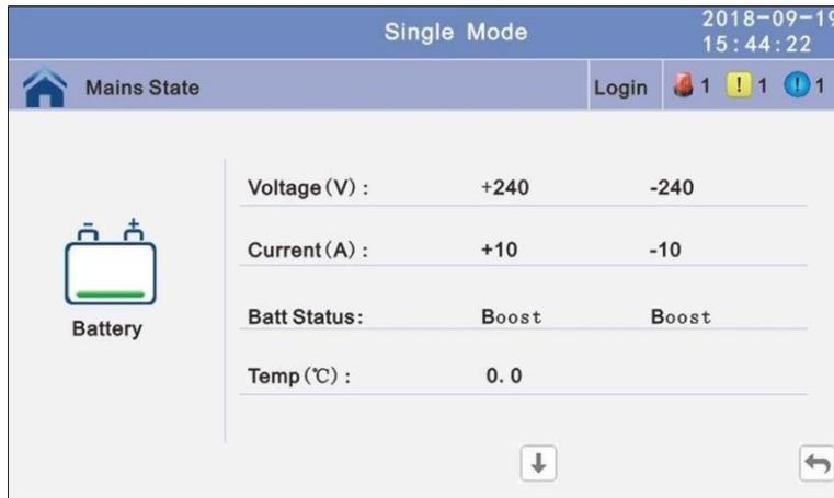
Fig. 4-9 Submenú Status/Battery (1)
