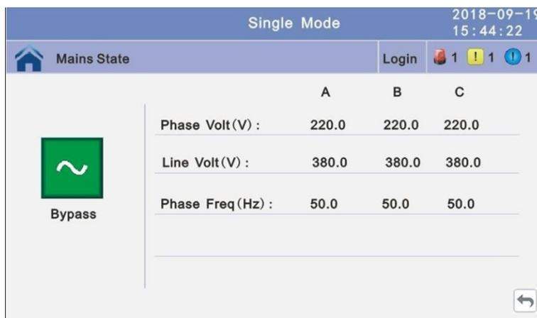
Fig. 4-6 Submenú Status/Bypass
