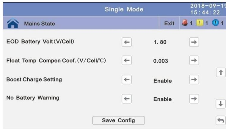
Fig. 4-38 Submenú Settings/Advanced Settings/System Setting (8)
