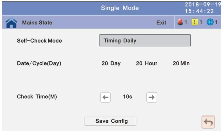
Fig. 4-52 Submenú Maint/Battery Self-Check/Timing daily
