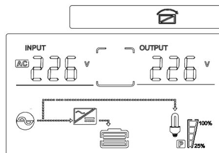
Fig. 4-4 Panel de control en modo bypass
